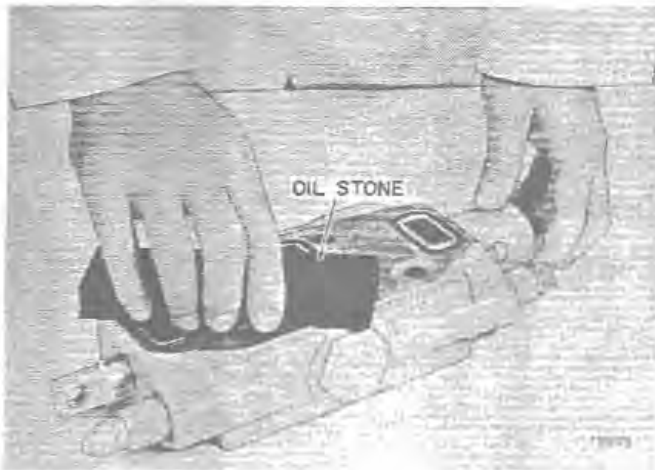
Figure 11 - Stoning a Valve Section
